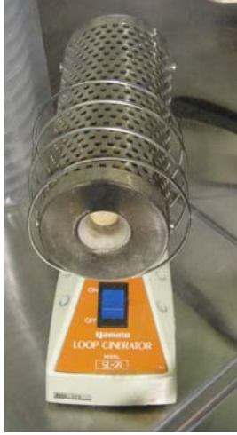
The loop incinerator
